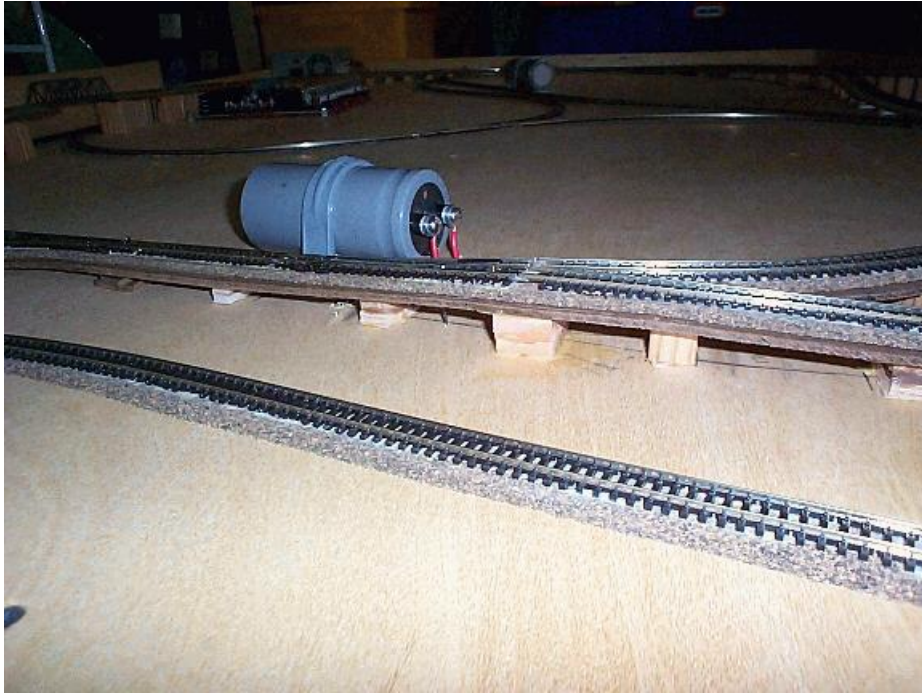
Figure 7 It is probably best to mount capacitor C16 somewhere on your baseboard rather than on the controller card itself
